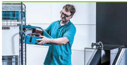
The Vertical Buffer Family units optimise your production logistics and guarantee continuous flow in the assembly area. Complete assembly sets can be retrieved just in time and conveyed directly to the assembly workstations. Compared to conventional shelving, throughput can be increased by up to 200%, depending on the application.
