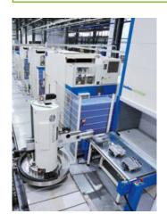
The full tray extraction feature was designed for the handling of heavy and bulky goods that often require the aid of a lifting device. Using full tray extraction, the tray is automatically pushed out onto an extraction table mounted to the front of the VLM for loading and unloading. Trays can also be loaded onto the optional transport cart for safe and easy handling.
