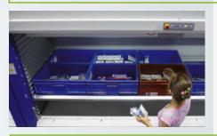
Side walls of the access opening are equipped with shelf rails, enabling the VLM to position more than one tray in the access opening. Also, individual users can adjust the delivery height of the tray to match their physical height providing true ergonomic working conditions.
