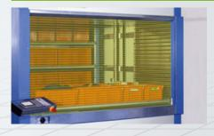
When the shutter doors open to deliver or retrieve a tray the safety light curtain located at the front of the access opening is activated. If the safety light barrier in front of the access opening is interruped, all movement of the device is stopped immediately for operator safety.
