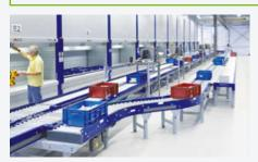
For quick picking and consolidation of orders, the connection of work zones via conveyor systems is an ideal solution. Items are delivered automatically to the access opening, picked and then placed into shipping containers on the conveyor.
