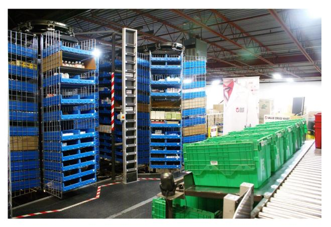
The carousels are an efficient way to pick goods because they rotate to bring the goods that need to be picked to the picker, while Power Pick Global controls the carousels and manages carousel inventory, is smart enough to coordinate batch picking as order requirements come down from the WMS.
