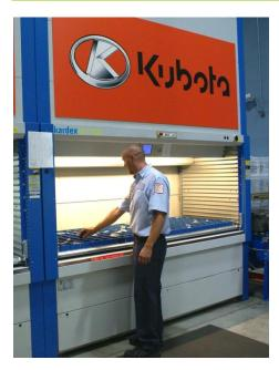
Much of the efficiency from AS/RS equipment comes from replacing substantial amounts of picker travel and handling with a high-density, "goods-to-person" environment in which one or two pickers at a workstation follow pick-to-light instructions to rapidly pick orders. Of course, in many DCs, goods from AS/RS zones need to join up with goods picked from other areas of the warehouse.
