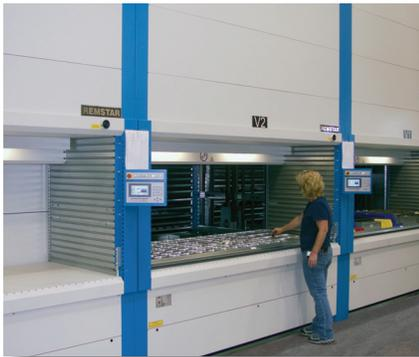
*The three Shuttle VLMs were installed in the workzones where the modules are built. With the shelving condensed into the VLMs the free floor space was used for a value generating module assembly area while the parts were kept close at hand.*
