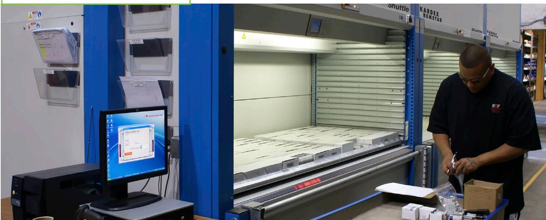
The warehouse was redesigned to include three Shuttle Vertical Lift Modules (VLMs) with pick to light technology integrated with Power Pick Global inventory management software. National Oilwell Varco-SHP Facility is now picking orders 44% faster using 27% less labor while recovering 70% of previously occupied shelving space.
